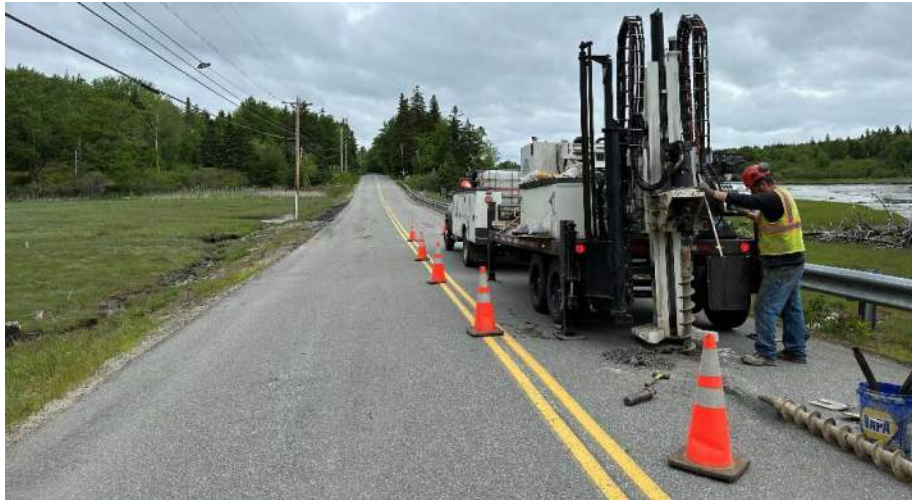
Drilling Test Boring B-1 (Facing North)
