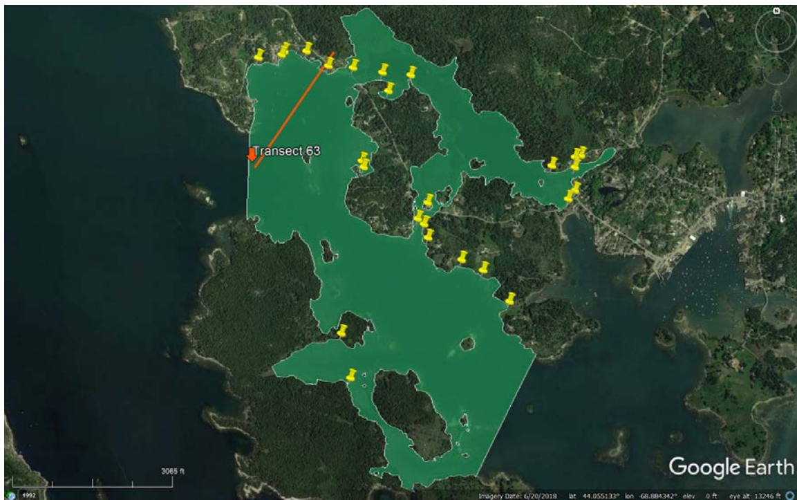
Figure 11: AE 12 Flood zone mapped based on Transect 63. Pushpins indicate buildings or roadways that are visible in the flood zone based on Google Earth imagery.
