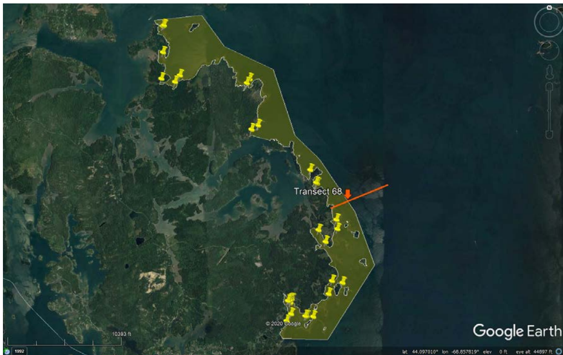
Figure 16. VE 22 Flood zone mapped based on Transect 68. Pushpins indicate buildings and roadways that are visible in the flood zone based on Google Earth imagery.
