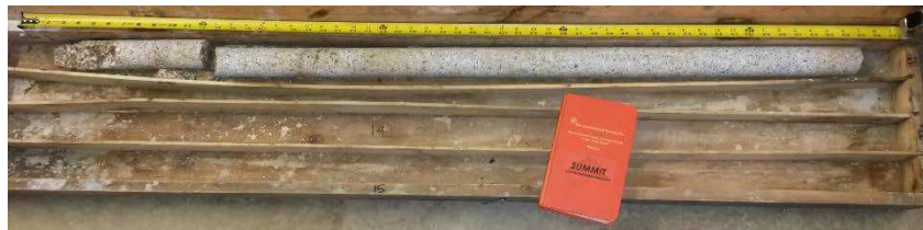
Boring B-2 (3.5 to 8.5 feet) – Rock Core (Granite)
