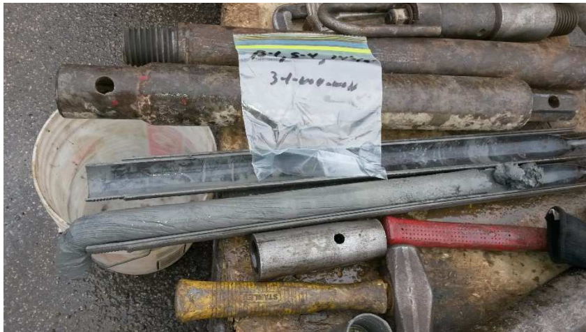
Boring B-1 (14 to 16 feet) – Marine Deposit (Gray Clay)
