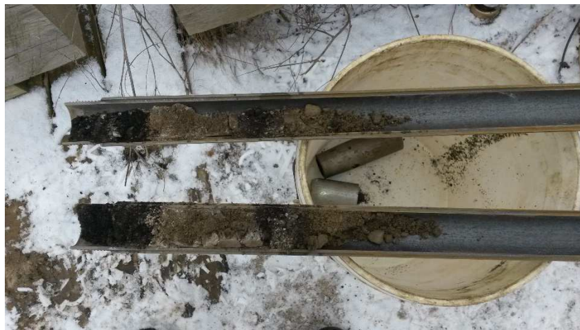
Boring B-1 (0.5 to 2.5 feet) – Granular Fill (Gravelly Sand w/Ash)
