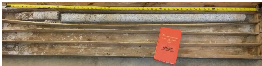
Boring B-2 (3.5 to 8.5 feet) – Rock Core (Granite)
